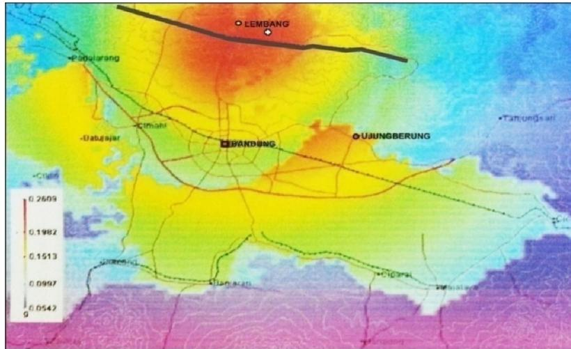
**Figure 1 Potential Maximum Peak Ground Acceleration by Lembang Fault Earthquake**
