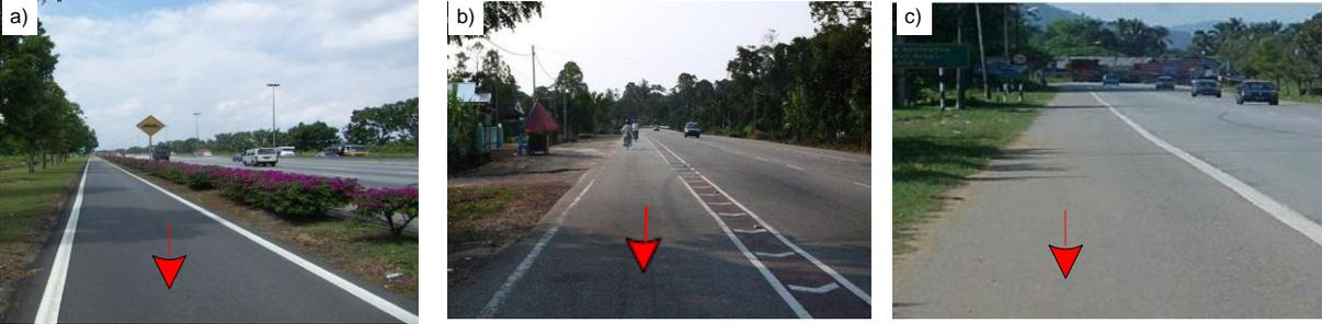
Figure 2 Illustrations of: a) an exclusive road lane, b) an inclusive road lane, and c) a paved shoulder road lane
